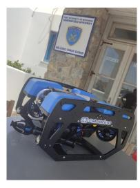
providing vessels with underwater monitoring capacity and also pollution monitoring. It is able to transmit real-time, high-quality video from areas that divers are unable to visit, with a span of up to 100 meters. It will be made available also to all neighboring islands if need be.
